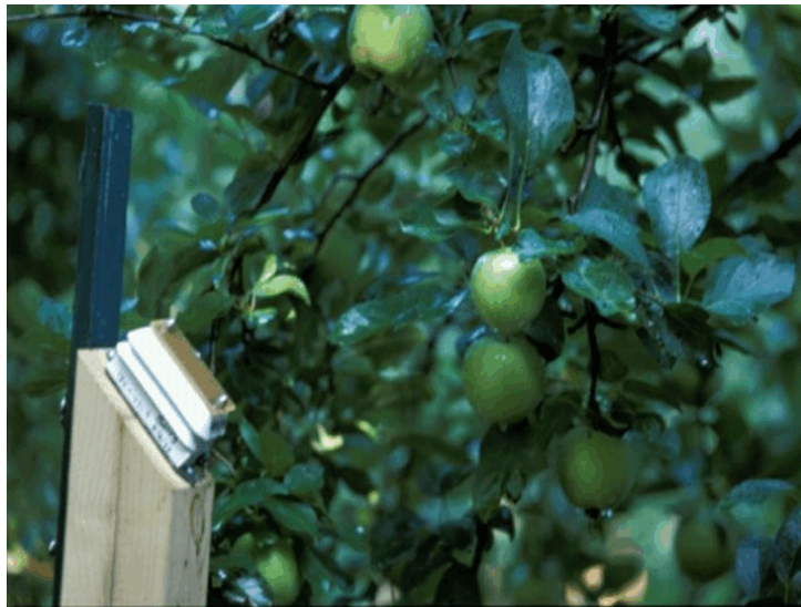
Figure 5. A Wetness/Temperature Logger under canopy of an apple tree.
